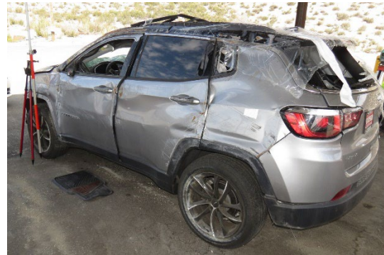
Figure 2. 2018 Jeep Compass, rollover damage
