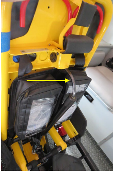
Figure 17. Bent pneumatic piston for back support adjustment denoted by the yellow arrow
