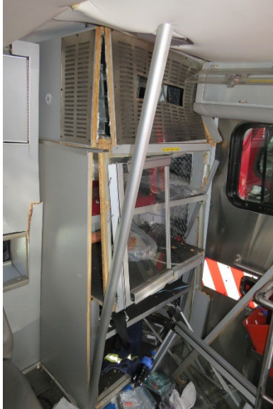
Figure 11. Damaged right front cabinets
