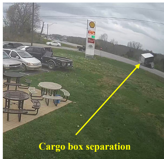
Figure 6. Video surveillance of impact, truck/ cargo box separation from truck frame (ambulance is under truck). Image used with permission.
