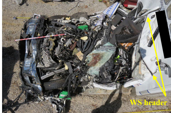
Figure 7. Overhead view of front end/cab damage (WS header noted for reference)
