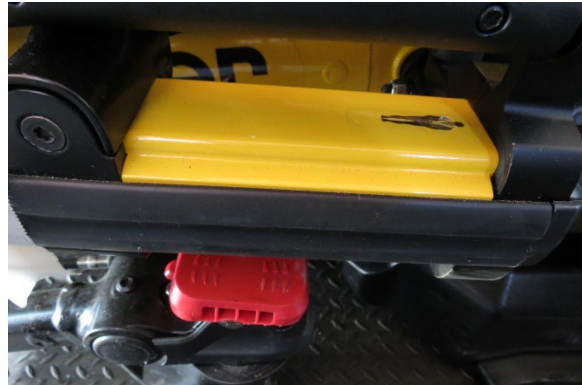
Figure 15. Proper mounting location for left shoulder restraint webbing
